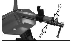
9. When ready to use, slide the handle (5) into the breaker arm. At other times it can be stored in the socket on the side of the base assembly.
